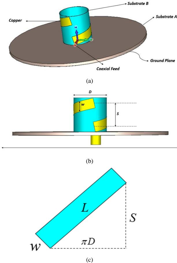
Figure 1: The structure of the proposed antenna: (a) 3D view, (b) Side view, and (c) unrolled strip helix of one turn.
