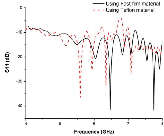
Figure 7: Comparison of 5.6 GHz helical antenna using fast-film and Teflon material
