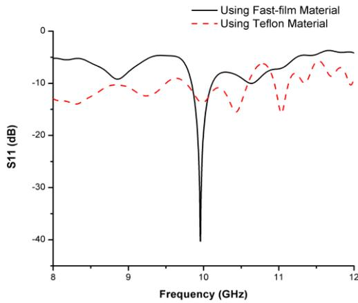
Figure 3: Comparison of 10 GHz helical antenna using fast-film and Teflon material
