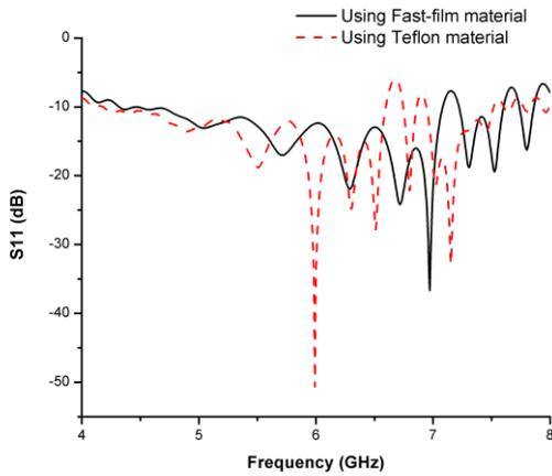
Figure 6: Comparison of 5.8 GHz helical antenna using fast-film and Teflon material
