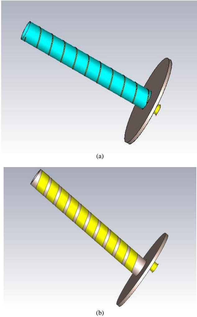
Figure 2: Design structure of 10 GHz Helical Antenna: (a) using fast-film material, (b) using Teflon Material
