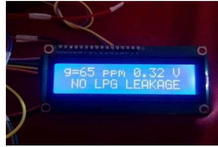
Figure 5: The gas concentration and voltage range displayed on the LCD.
