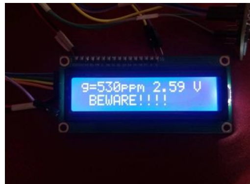
Figure 7: The gas concentration and voltage range that display on the LCD.
