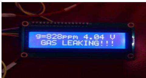
Figure 10: The gas concentration and voltage range displayed on the LCD.
