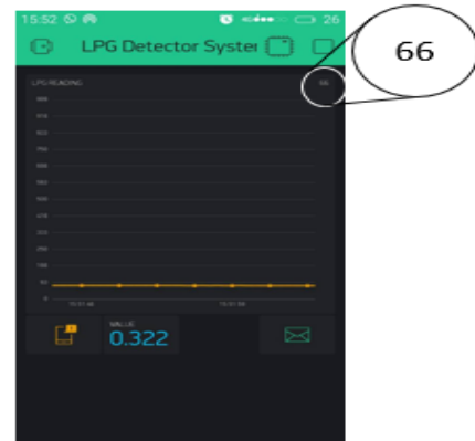
Figure 6: The gas concentration and voltage range displayed graphically on the Blynk application.
