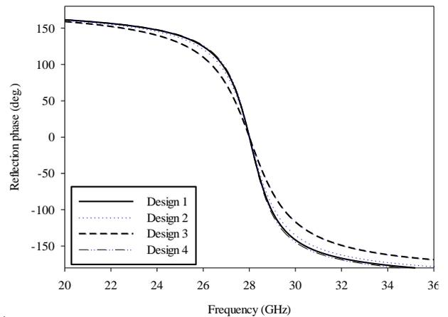
Figure 2: Reflection phase of proposed design AMCs
