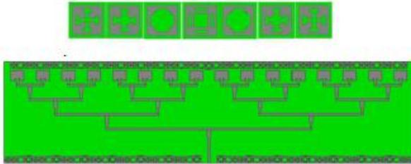
Figure 4: 16x1 antenna array with non-periodic AMCs 1
