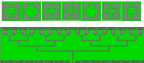
Figure 5: 16x1 antenna array with non-periodic AMCs 2
