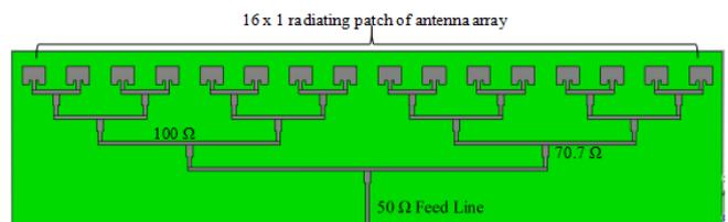
Figure 3: 16x1 antenna array without AMC structure
