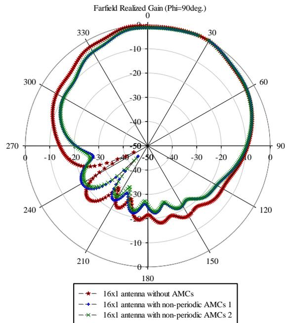
Figure 7: The gain of the antenna without and with AMC structures
