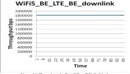
Figure 16: Throughput for Best Effort (BE) QoS both for LTE and Wi-Fi network
