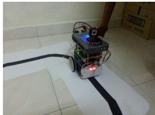
Figure 7: Prototype robot missed the track at the corner but back to the line after that.
