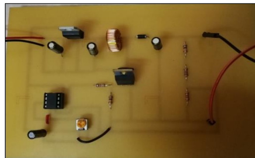
Figure 8: The Hardware Circuit of the Voltage Regulator and Boost Converter Using ATtiny85.
