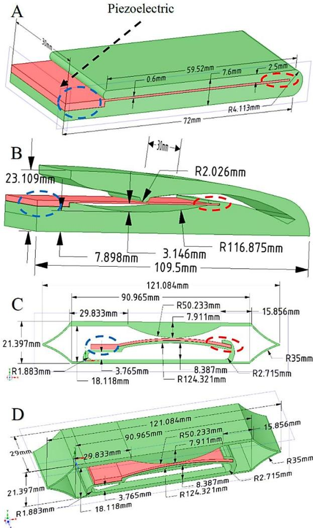
Figure 2: 3D models of the proposed piezoelectric bending mechanisms where, A: Flat Mechanism, B: Unstressed Mechanism, C and D: Pre-stressed mechanism.
