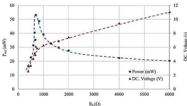
Figure 8: Direct power and voltage at varying load.
