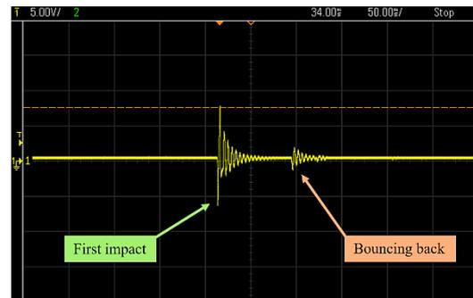
Figure 6: DSO screenshot capturing the piezo output voltage waveform at the open - circuit when it's been impacted at specific force.
