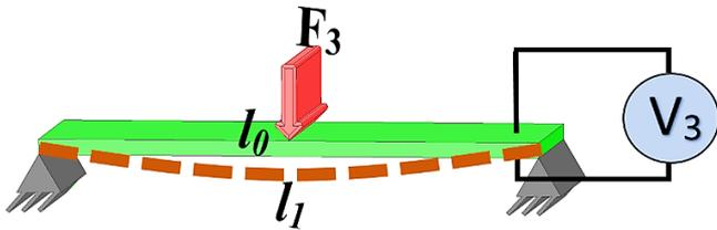
Figure 1: Applying  $F_3$  will lead to stress the piezoelectric material by  $l_1$  and generate an electrical signal  $V_3$ .
