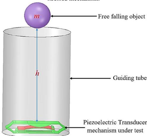
Figure 5: Drop test experiment set-up.
