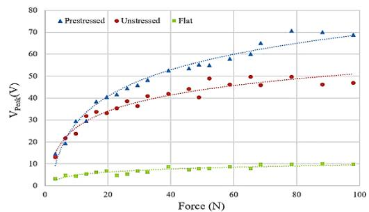
Figure 7: AC. V recovered via the piezoelectric transducer bending mechanisms that been impacted at varying forces.
