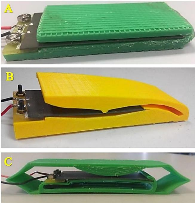
Figure 4: 3D printed prototypes that used to conduct the evaluation phase where, A: Flat Mechanism, B: Unstressed Mechanism, C: Pre-stressed mechanism.
