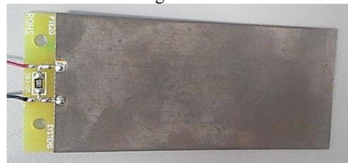
Figure 3: Piezoelectric transducer.
