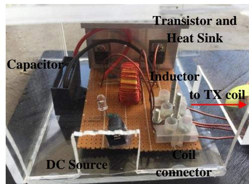
Figure 4: Hardware implementation of the transmitter circuit
