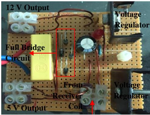
Figure 5: Hardware implementation of the receiver circuit
