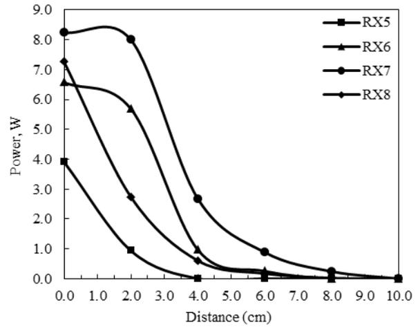
Figure 11: Output power over distance using TX1 ( $D_{T2} = D_{R2} = 9.5$  mm).
