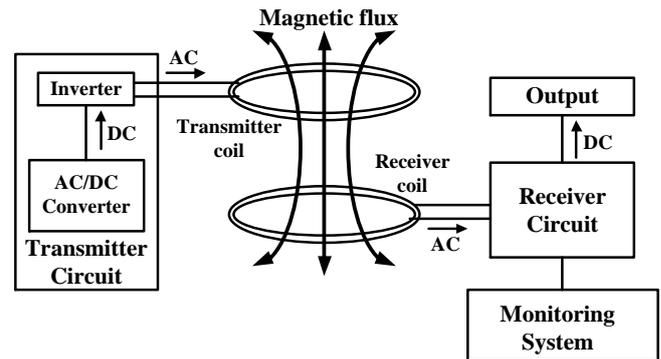
Figure 3: Block diagram of a wireless power transfer
