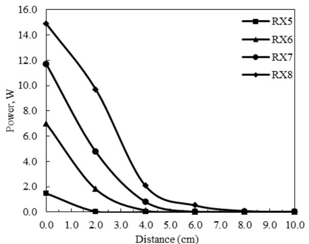
Figure 13: Output power over distance using TX3 ( $D_{T2} = D_{R2} = 9.5$  mm).
