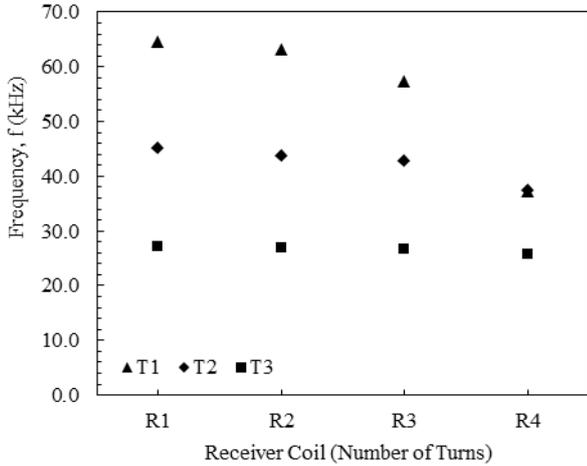
Figure 9: Characteristics of resonant frequency for transmitter-receiver coils pairs ( $D_{T1} = D_{R1} = 6.5$  mm)
