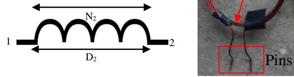
Figure 2: Receiver coil (RX) dimension
