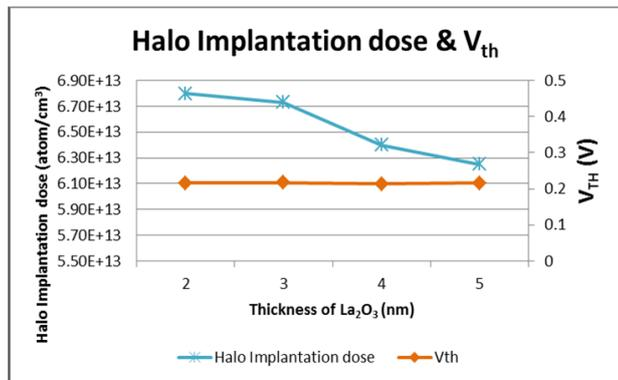
Figure 8: Graph of Halo Implantation dose and threshold voltage ( $V_{TH}$ ) for different  $La_2O_3$  thicknesses
