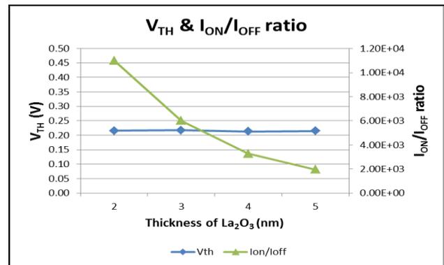
Figure 6: Graph of threshold voltage ( $V_{TH}$ ) and on/off current ratio ( $I_{ON}/I_{OFF}$ ) for different  $La_2O_3$  thicknesses
