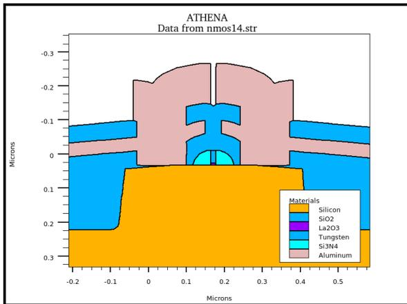
Figure 1: Structure of 14nm NMOS
