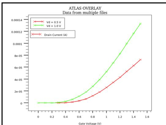
Figure 4: Graph of Drain Current( $I_D$ ) versus Gate Voltage( $V_G$ )
