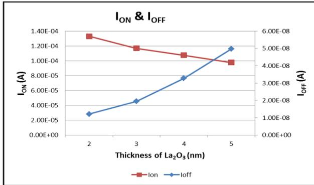
Figure 7: Graph of on-current ( $I_{ON}$ ) and off current ( $I_{OFF}$ ) for different  $La_2O_3$  thickness
