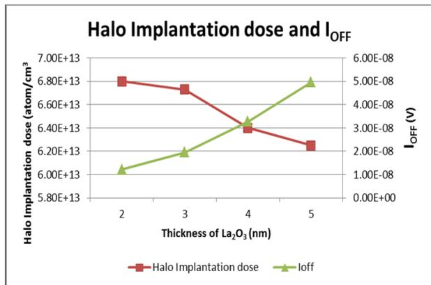
Figure 9: Graph of Halo Implantation dose and off-current ( $I_{OFF}$ ) for different  $La_2O_3$  thickness
