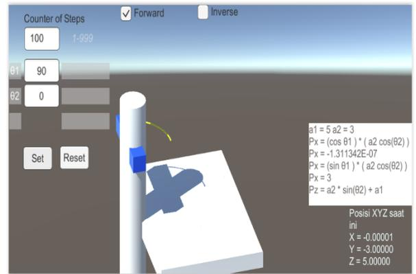
Figure 5: Forward kinematic result of 2 DOF robot using designed application software
