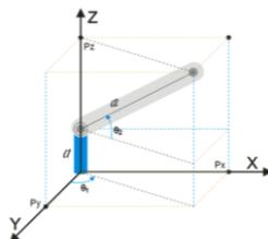
Figure 1: Robot model in 2 DOF coordinate system
