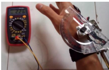
Figure 7: Measurement the arm angle and the output voltage of the sensor
