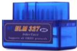
Figure 4: OBD-II dongle with the ELM327 integrated circuit and Bluetooth connection
