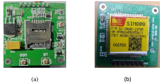
Figure 3: (a) Bottom side of SIMCOM808 with GSM slot, (b) Top side of SIM808 module.
