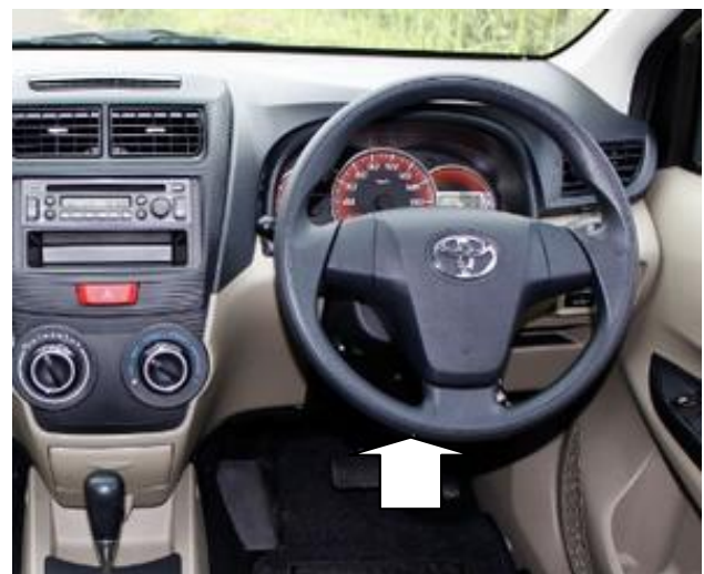
Figure 1: Illustration of the location of OBD-II connector indicated by arrow
