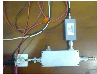
Figure 3: Experimental setup for measuring S_{11}
