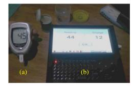
Figure 4: (a) Prototype vs (b) Glucose Meter Glucose Solution Reading
