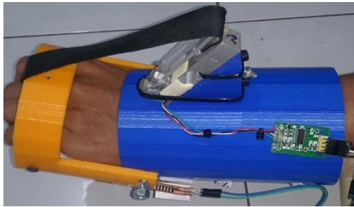
Figure 8: Wrist flexion exerciser prototype during a mock training session
