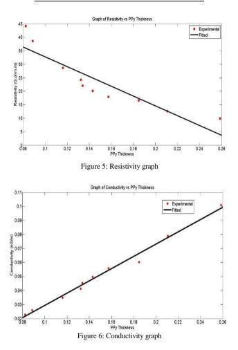
Table 3 shows the results of average electrical resistivity and average electrical conductivity which were determined for PPy thin films of different thicknesses. Figure 3 shows the plot of resistivity as a function of film thickness. The resistivity decreases when films thickness increases. It was also observed that as the PPy thin film increases, the conductivity increases thus suggesting that the deposited thin
