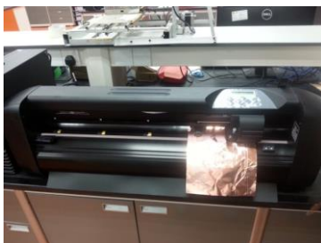
Figure 8: Process of circuit cutting using a vinyl cutter (Summacut D60R)
