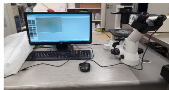
Figure 5: Nikon TS100 inverted microscope with Dino camera and Dinocapture2.0 Software
