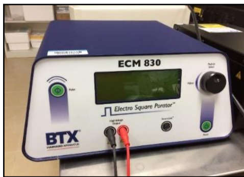
Figure 2: ECM@830 square wave pulse generator
