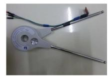
Figure 5: Goniometer with Accelerometer.
