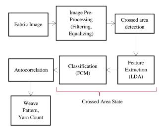
Figure 2: Block Diagram of Automatic Woven Structure Recognition
