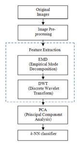
Figure 1: The block diagram of the proposed method
