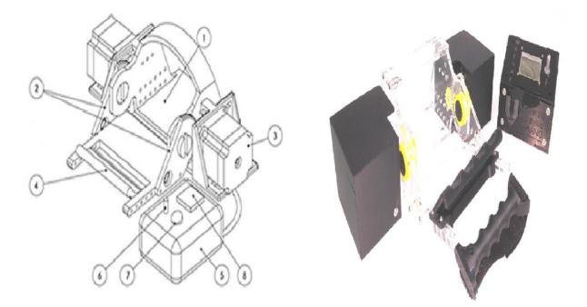
Figure 1: *Right*-Illustrated an embodiment of the WRist-T device. *Left*-The prototype of the wrist rehabilitation therapy (WRist-T) device. Notes: Description of the reference numerals used in the accompanying drawings according to the WRist-T device; (1) channel; (2) platform arm; (3) motor; (4) hand support; (5) controller; (6) toggle switch; (7) power button; (8) LCD display.
