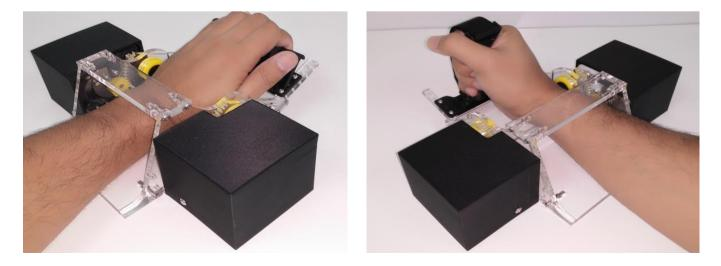
Figure 4: A 3D printed prototype of WRist-T device tested to an ischemic stroke patient. The figure shows details the example wrist of motion on extension/flexion and radial/ulnar deviation exercise.
