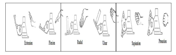
Figure 2: A perspective views of the device in an embodiment to give (a) Motion forextension/flexion; (b) Radial/ulna deviation; and (c). Supination/pronation of the wrist.
