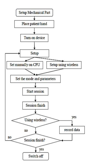
Figure 3: The flowchart of the WRist-T device function.
