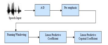
Figure 2: Block diagram of Linear Predictive parameter
