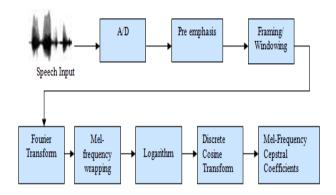
Figure 3: Block diagram of Mel-Frequency Cepstral Coefficient
