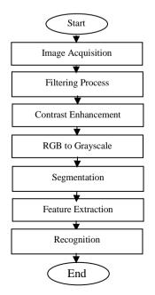
Figure 1: Flowchart of an Intelligent Recognition
