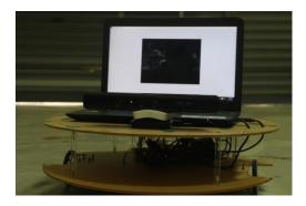
Figure 7: The mobile scanner
