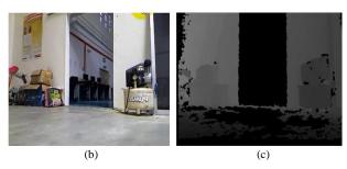
Figure 9: (a) Position of the platform in scanning scene 3; (b) The resulting scan of scene 3 in the image; (c) The resulting scan of scene 3 in-depth data
