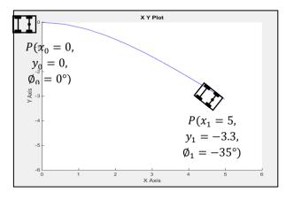
Figure 17: Forward right parking plotted in XY-graph
