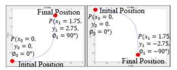
Figure 7: Graph for forward left (1) and right (2) motion
