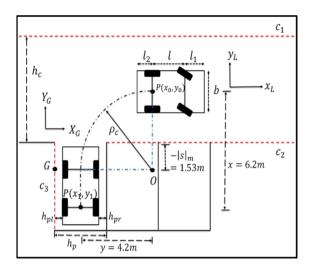
Figure 5: Geometry of perpendicular reverse right
