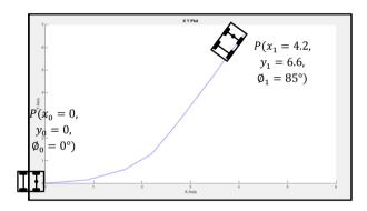
Figure 13: Forward left parking plotted in XY-graph
