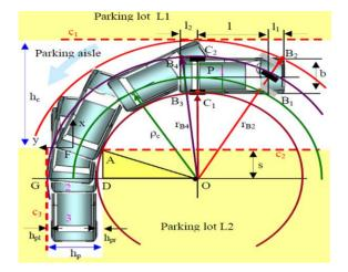
Figure 3: Geometry of collision-free reverse perpendicular parking manoeuvre [5]
