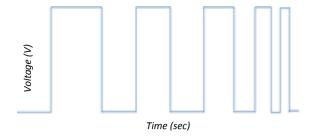
Figure 9: PWM input signal for segment B (acceleration)
