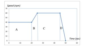
Figure 7: Desired conching process output profile.
