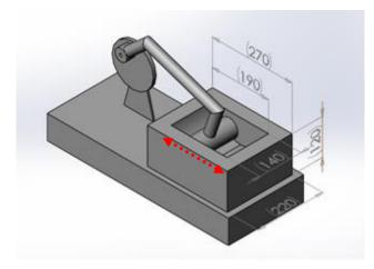
Figure 2: Dimensions (in mm) of the rig
