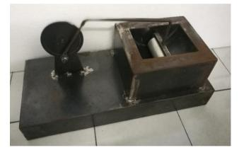
Figure 1: The designed test rig for dodol conching process.
