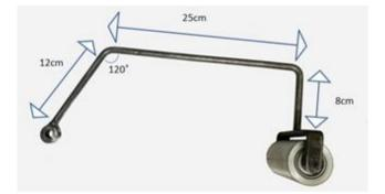
Figure 3: Dimensions of the roller arm
