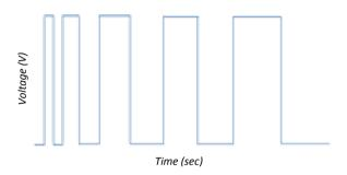
Figure 11: PWM input signal for segment D (deceleration)
