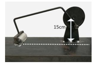
Figure 5: Height or location of the roller from the centre of driving disc.
