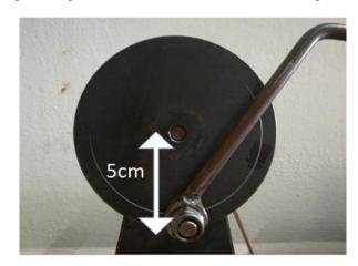
Figure 6: Distance between the joint of roller arm to the centre point of driving disc.
