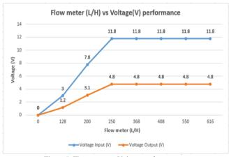
Figure 5: Flow meter vs Voltage performance
