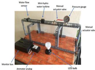
Figure 2: Residential piping designed system
