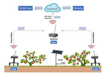
Figure 4: The Operation of the System
