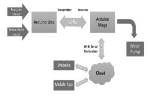
Figure 3: The Overall Block Diagram of the System
