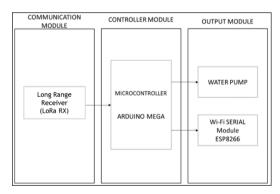
Figure 2: Receiver (Base) Block Diagram of the System
