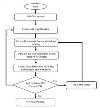
Figure 5: Automatic Irrigation Monitoring System Using Android Based Application Algorithm
