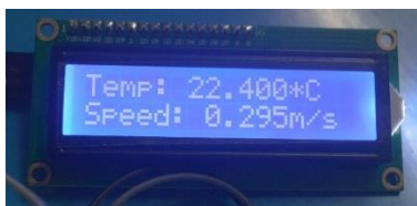
Figure 6: Display of the air temperature and air velocity when PMV index of +0.5 is selected
