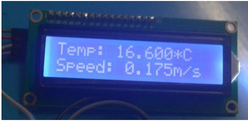
Figure 10: Display of the air temperature and air velocity when PMV index of -1 is selected.
