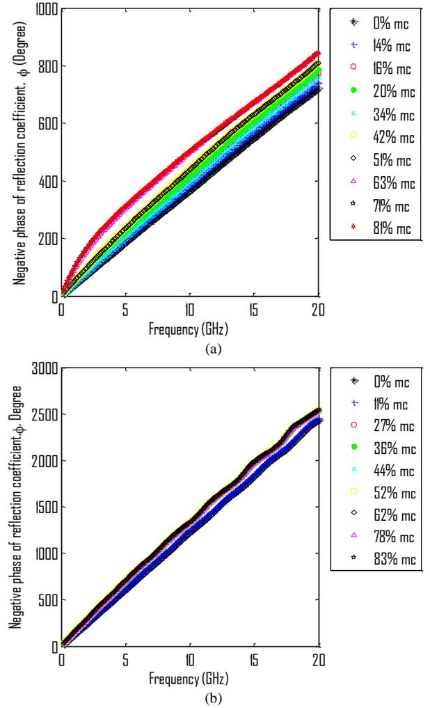
Figure 3: The variation of measured negative phase,  $\phi$  with frequency using (a) open-ended coaxial probe and (b) Agilent 85070E High Temperature Probe for different moisture content (mc) in beef.
