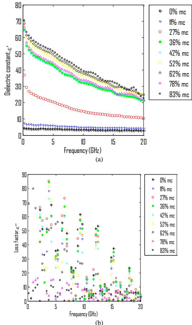
Figure 1: Frequency response of (a) dielectric constant,  $\epsilon'$  and (b) loss factor,  $\epsilon''$  with various  $mc$ .
