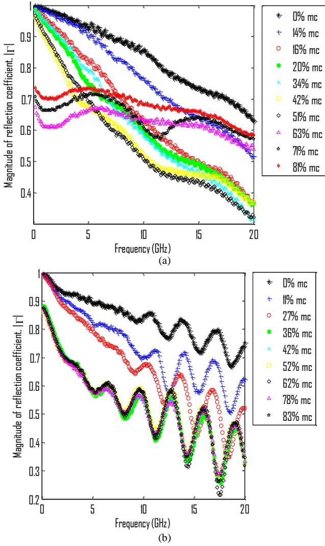
Figure 2: The variation of measured  $|Γ|$  with frequency using (a) open-ended coaxial probe and (b) Agilent 85070E High Temperature Probe for different moisture content (mc) in beef.
