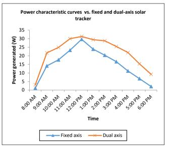
Figure 9: Solar tracking systems power generated
