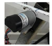
Figure 6: DC motor in place
