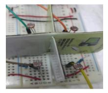
Figure 7: The arrangement of LDR sensors
