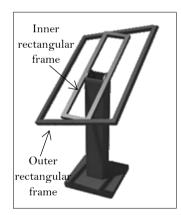
Figure 2: The 3D model of a dual axis solar tracking system
