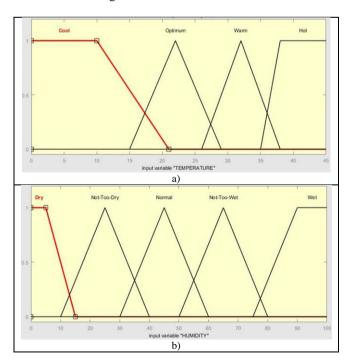
Figure 9: Input variable; a) Temperature with four membership function; b) Humidity with five membership function
