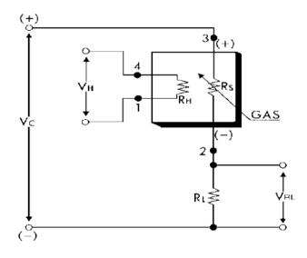
Figure 4: MOS gas sensor circuit diagram
