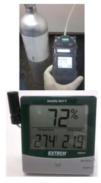
Figure 7: Altair 5x Multi Gas Detector and Humidity Alert II
