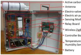
Active carbon filter Electric air pump Sensing Module Wireless ZigBee Controller Board Temperature & Humidity Sensor
