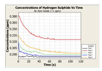
Figure 11: Graph of H<sub>2</sub>S concentrations (<1 ppm) versus time
