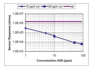
Figure 5: Graph of hydrogen sulphide (H<sub>2</sub>S) sensor response versus concentrations
