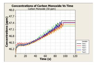
Figure 9: Graph of CO concentrations (50 ppm) versus time
