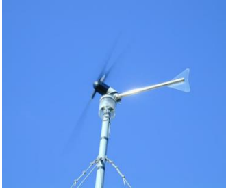
Figure 2: Furling mechanism (Photo courtesy of NREL - Dean Davis.)
