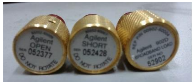
Figure 3: Calibration standards of Open, Short and Broadband Load
