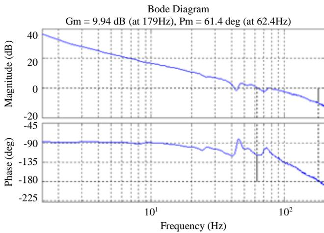
Figure 2: Gain Margin and Phase Margin
