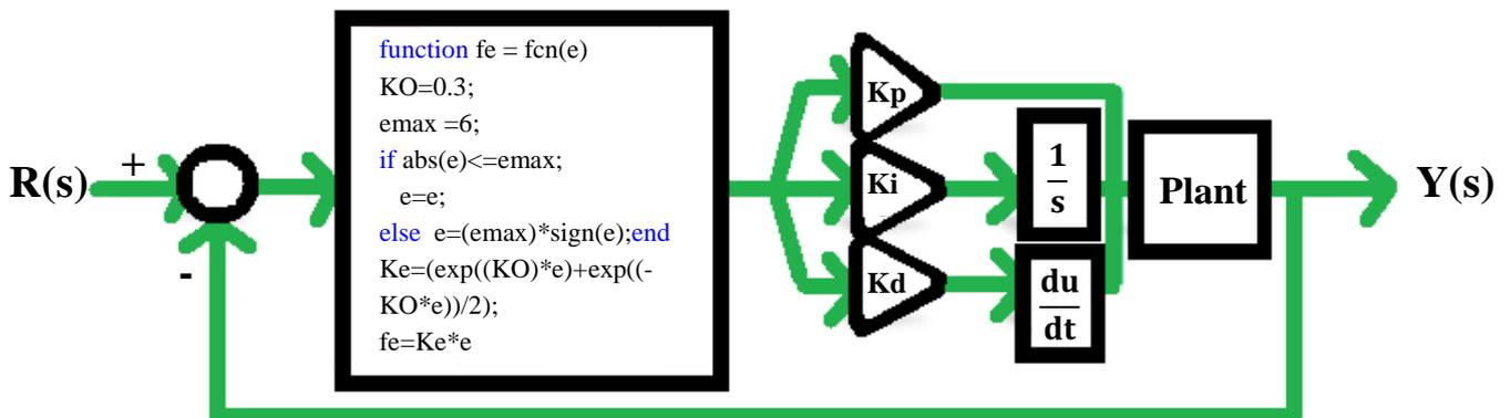
Figure 9: Design of NPID based on  $K(e)$
