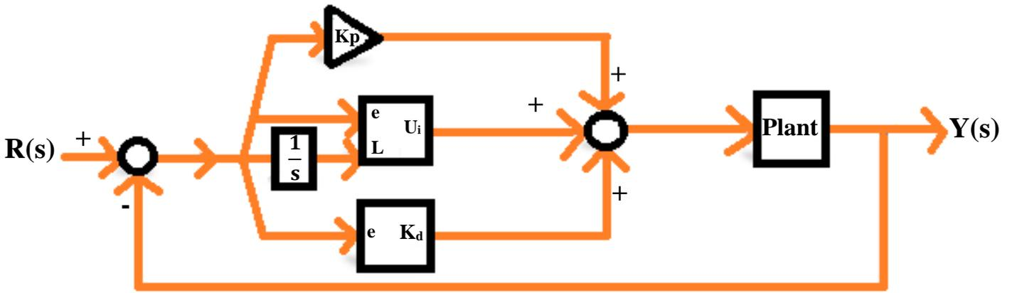
Figure 7: Design of NPID based on  $U_i$  and  $K_d$
