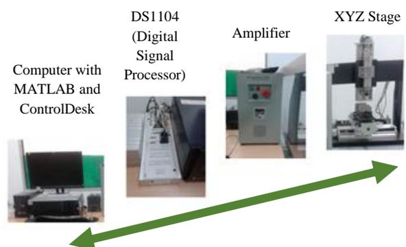
Figure 1: Experimental setup of ball screw drive
