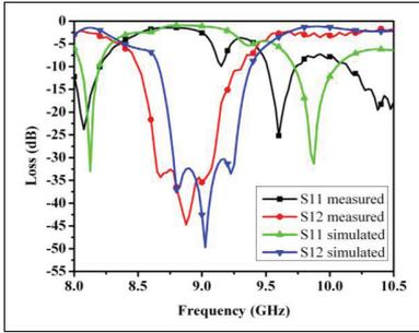
Figure 6 Simulated and measured responses of the transmission mode substrate-integrated-waveguide bandstop filter.
