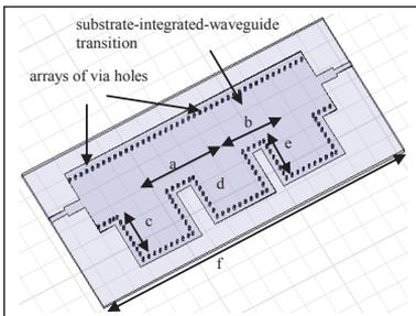
Figure 4 Three-stage transmission substrate-integrated-waveguide bandstop filter ( $a=18.8$  mm,  $b=17.4$  mm,  $c=10.5$  mm,  $d=9.7$  mm,  $e=9.2$  mm,  $f=58.5$  mm, diameter of via hole=0.5mm, distance between adjacent via holes=1.0 mm).
