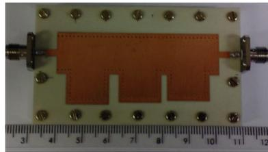
Figure 5 Manufactured transmission mode substrate-integrated-waveguide bandstop filter.
