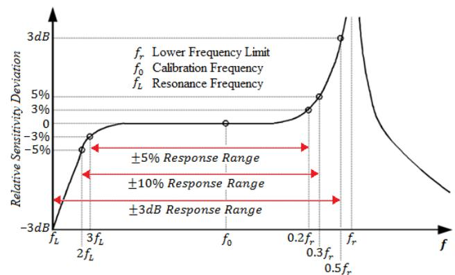
Figure 1. Frequency Response Curve [5]
