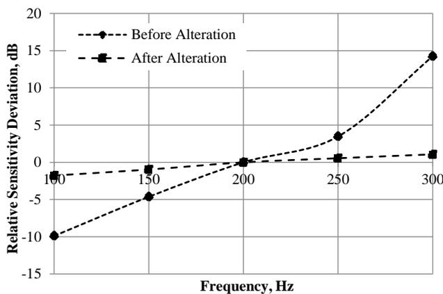
Figure 9. Frequency Response Curve for CL Before and After Alteration.
