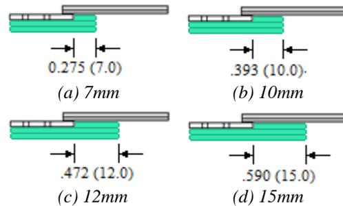
Figure 4. Illustration for Reducing Cantilever Length by Clamping Over
