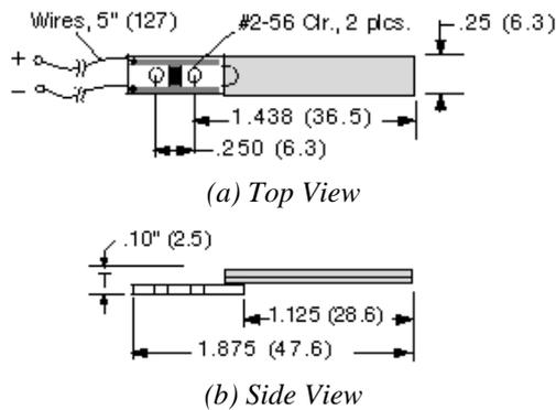
Figure 2. Dimension of Piezoelectric Cantilever (Q220-A4-203YB) [6].
