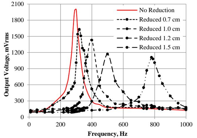
Figure 7. Frequency Response of the Cantilever after Length Reduction.
