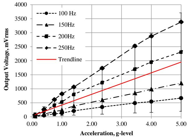
Figure 6. Output Voltage obtained under Variation of Acceleration Level with Trendline and Deviation Bar.
