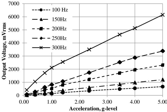
Figure 5. Output Voltage obtained under Variation of Acceleration Level.
