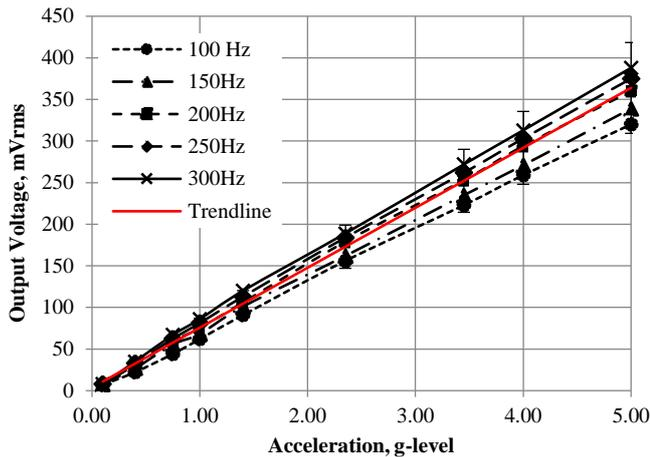
Figure 8. Output Voltage obtained under Variation of Acceleration Level after Resonant Frequency Alteration with 1.5 cm cantilever length reduction.
