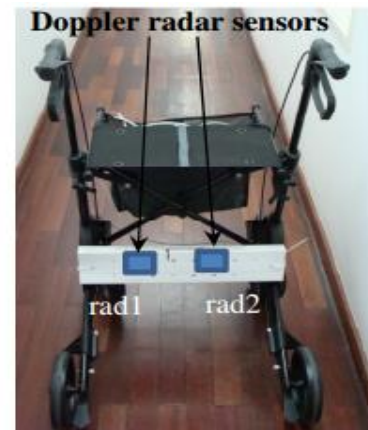
Figure 4: Four wheels walker with 2X FMCW Doppler radar [17]
