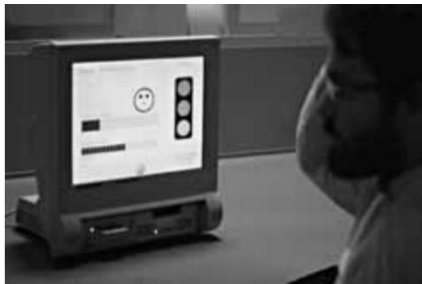
Figure 18: The feedback interface. Traffic lights signal the start of an exercise; bars grow to show progress; the face smiles or frowns depending on the correctness of the execution [20]
