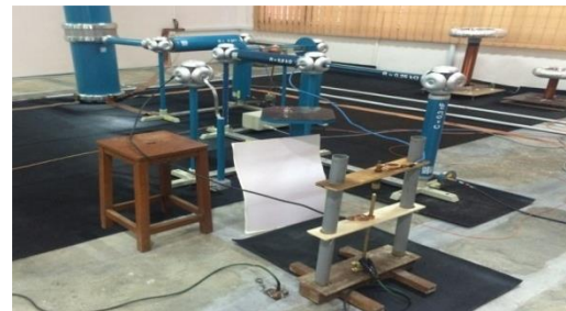
Figure 2: Experimental setup for lightning impulse voltage test
