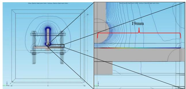
Figure 10: Electric field pattern with polyimide material in CIGRE Method II Electrode Configuration
