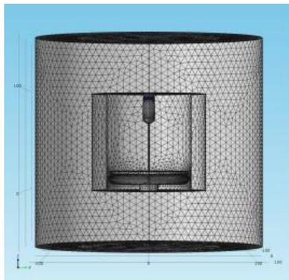
(b) Mesh analysis of point to plane electrode test cell
