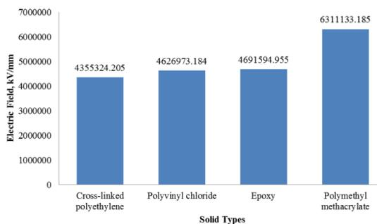
Figure 12: Maximum Electric Field at 50kV
