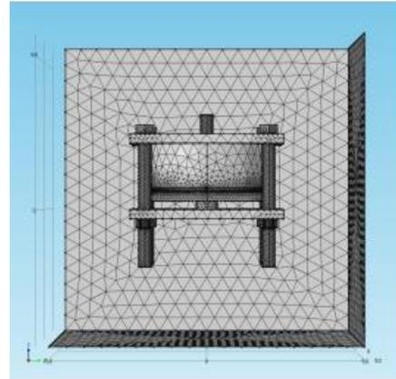
(b) Mesh analysis of CIGRE Method II electrode configuration
