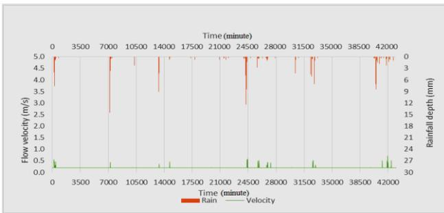
Figure 5: Variation of Flow Velocity with Rainfall Events for September 2009
