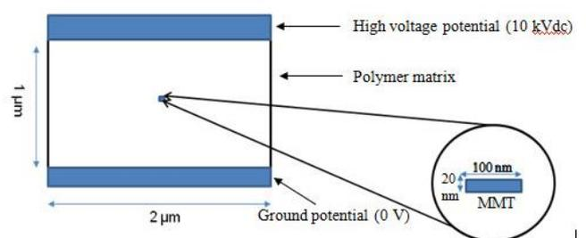
Figure 1: A two dimensional slab with thickness 1  $\mu\text{m}$  and width 2  $\mu\text{m}$  was placed between 10 kV DC high voltage (HV) potential and 0 V ground potential.
