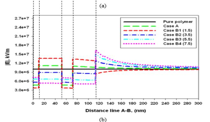
Figure 4: Effect of (a) nanoparticle (with separated 40 nm apart) on the (b) plots of the electric field intensity along the line AB from the origin
