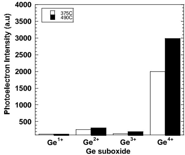
Figure 3: Signal intensity of deconvoluted Ge oxide components (Ge<sup>1+~4+</sup>) for thermally grown Ge oxide/Ge(100) at 375 and 490 °C measured at take-off angle of 30°
