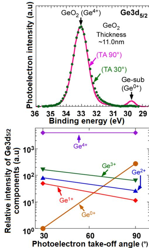
Figure 7 Take-off angle dependence of  $\text{Ge}/\text{GeO}_2$  stack after anneal at temperature of  $375^\circ\text{C}$
