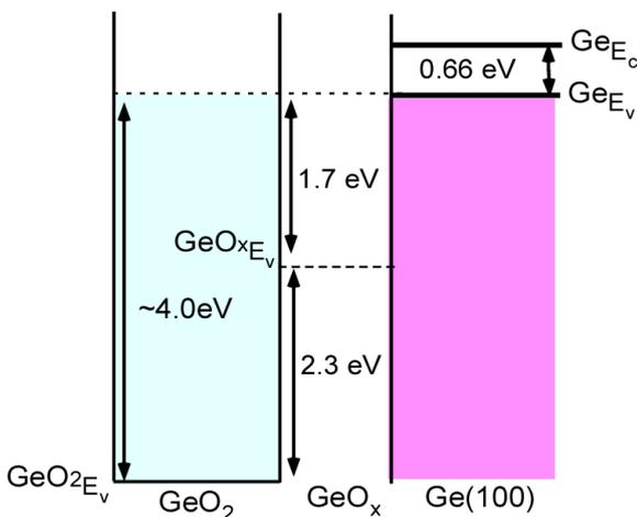
Figure 6: Energy band diagram of 11.0 nm-thick  $\text{GeO}_2$
