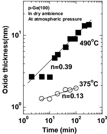
Figure 1: Thermal oxidation at temperature of 375 and 490 °C
