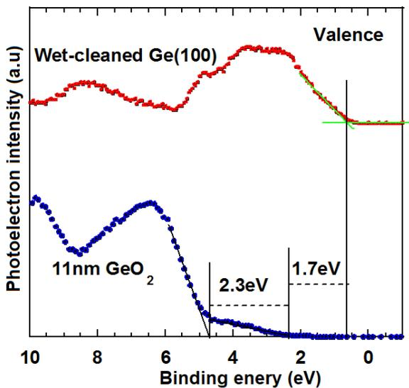
Figure 5: Valence band of 11.0 nm-thick Ge oxide
