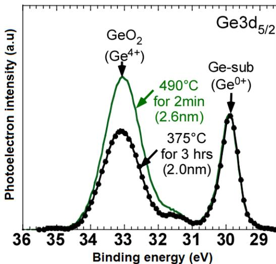
Figure 2: Ge 3d<sub>5/2</sub> spectra of thermally grown Ge oxide on Ge(100) surface at 375 and 490°C
