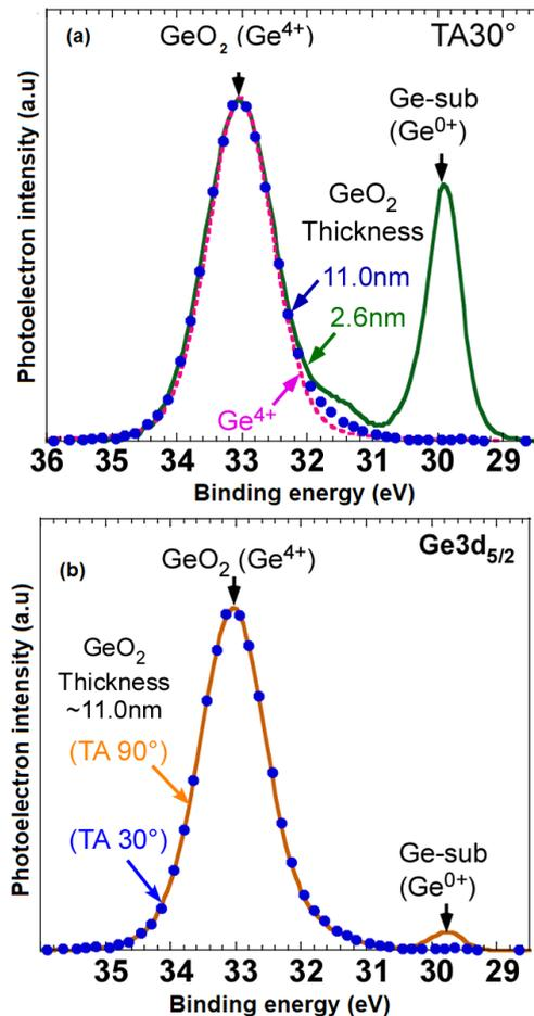
Figure 4: The thickness and takeoff angle dependence of GeO<sub>2</sub>
