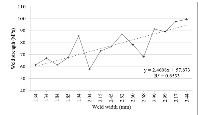
Figure 1: Joint strength versus joint width for laser joining of PET and 316L stainless steel.
