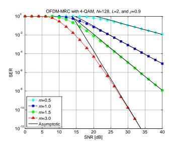
Figure 2: SER vs. SNR of OFDM-MRC with 4-QAM, N=128, L=2,  $\rho=0.9$ ,  $m=\{0.5, 1.0, 1.5, 3.0\}$  in correlated Nakagami-*m* fading channels
