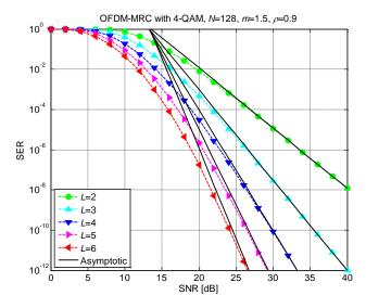
Figure 4: SER vs. SNR of OFDM-MRC with 4-QAM, N=128, m=1.5,  $\rho=0.9$ ,  $L=\{2, 3, 4, 5, 6\}$  in correlated Nakagami-*m* fading channels
