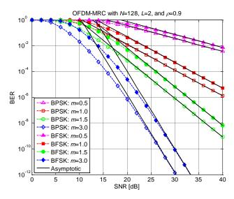
Figure 1: BER vs. SNR of OFDM-MRC with BPSK/BFSK, N=128, L=2,  $\rho=0.9$ ,  $m=\{0.5, 1.0, 1.5, 3.0\}$  in correlated Nakagami-*m* fading channels
