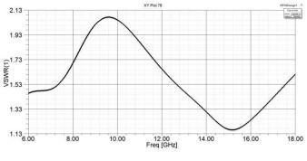
Figure 5: VSWR of unidirectional antenna
