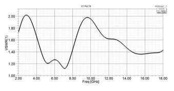
Figure 4: VSWR of bidirectional antenna
