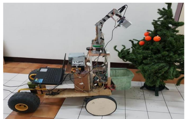
Figure 1: Autonomous Fruit Harvester with Machine Vision
